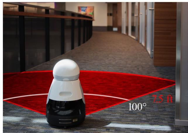
Fig. 1. Kuri in the halls of our academic building. Kuri is an expressive and engaging robot with low sensing and computation capabilities. Its lidar can only see up to 7.5 ft, insufficient to localize in long, wide hallways. Further, a significant portion of its compute gets used by localization algorithms. Motivated by these limited capabilities, in this paper we describe a system for “wandering” that enabled Kuri to traverse our large hallways for four days.
